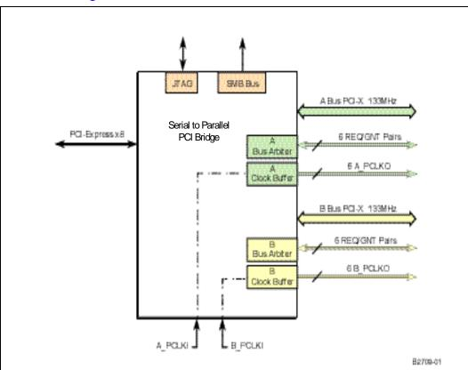
Figure 3. 41110 Block Diagram
